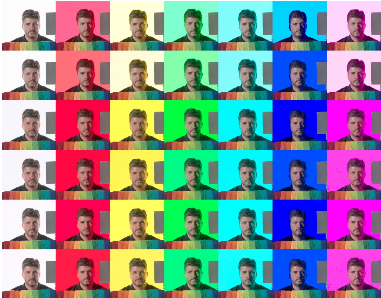
Figure 9 - Examples of hue-preserving viewing transform alternatives, from top to bottom, RDD 31, RDD 31 with hue_restore_dw3() [3] applied after the independent RGB tone curve and again after the AWG to BT.709 primary conversion, MaxRGB-norm, MaxRGB-norm with hue_restore_dw3() applied after AWG to BT.709 primary conversion, Power-norm (5ths over 4ths), Power-norm (5ths over 4ths) with hue_restore_dw3() applied after AWG to BT.709 primary conversion
