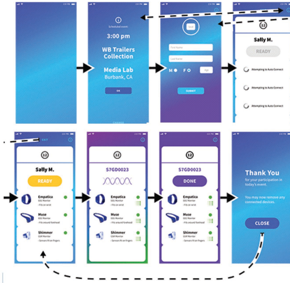
Figure 4: User Experience Flow. A user logs into their account via a wifi connection. The user selects a device to connect with via Bluetooth. Once connected the study begins and the content is displayed on a PC monitor.
